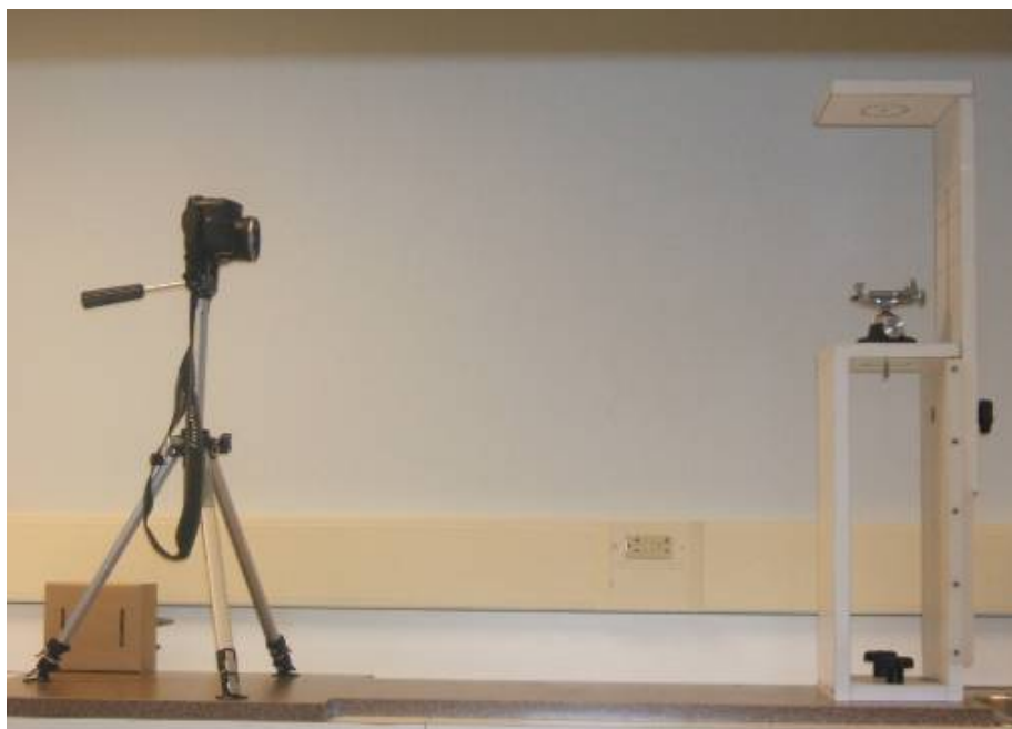
Figure 3.1: Measuring apparatus used to standardize model orientation
