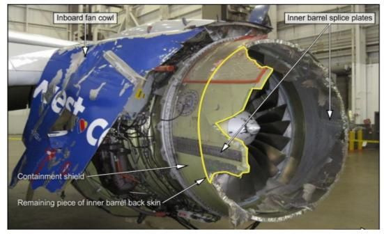
The disabled left engine by the broken fan blade
