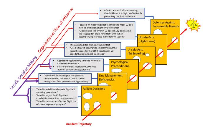
"Swiss Cheese" model applied to the Gulfstream G650 flight test accident at Roswell
