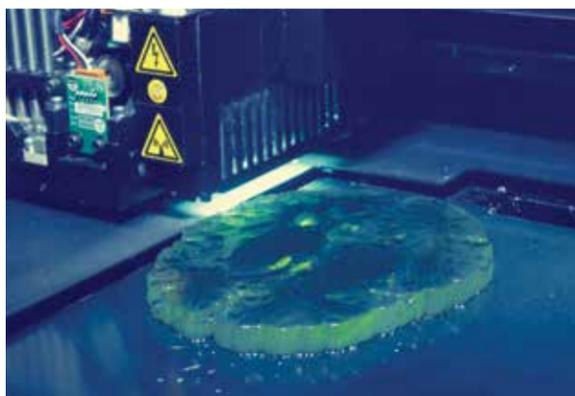
The 3-D organs are printed on a Stratasys Objet Eden 260VS printer in the Tinker Lab of Parks College. The printer works by printing the organ layer by layer in a resin or other durable material.
